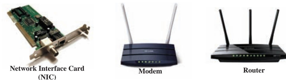
Figure 1.9 - Wired/Wireless Communication Devices
