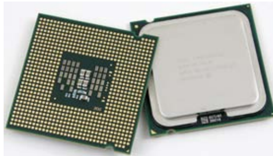
Figure 1.1 - Central Processing Unit
